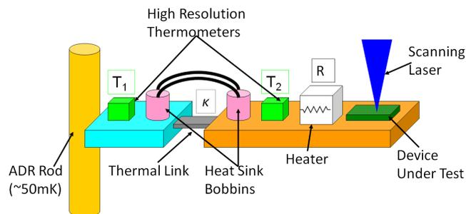
Fig. 3. Measuring absorbed power via thermometry. See text for details.
