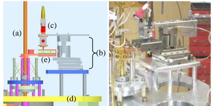
Fig. 1. The cold parts of the scanning pulser. Left: solid model view, showing: (a) vertical copper rod from the salt pill of the adiabatic demagnetization refrigerator, (b) XYZ scanning stage stack, (c) objective assembly, fiber optic connector shown at top, (d) 3 K flange, (e) shielded box holding detectors. Right: as implemented. A counterweight for the optical head reduces off-axis loading of the XYZ scanning stage.
